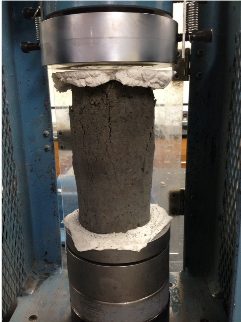
Figure 3-8. Gypsum Cement capped CLSM cylinder after failure.
