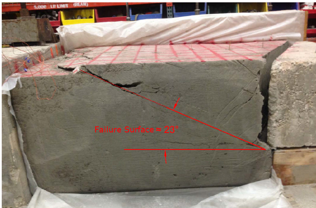
Figure 4-11. Failure surface profile.
