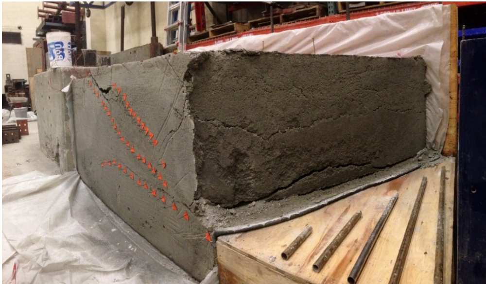
Figure 4-13. Isometric view of the failure planes.
